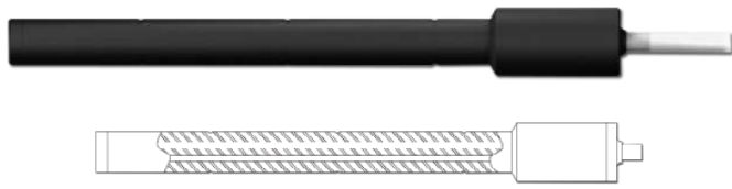
Exradin A17 Schematic
