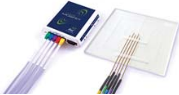
Calibration jig shown with mobileMOSFET
