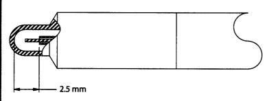
Centroid of Collecting Volume: 1.8 mm from tip of shell Outside Diameter of Shell Collecting Volume: 3.4 mm Collector Diameter: 0.3 mm x 1.27 mm length Shell Wall Thickness: 0.5 mm
