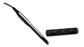
The Solid Water® Farmer Chamber is a 0.6 cm<sup>3</sup> volume ionization chamber, the standard for absolute dosimetry measurements in air, water or phantom material. The chamber is constructed entirely out of GAMMEX RMI's trademark Solid Water material with a central aluminum electrode. It is fully guarded up to the measuring volume and comes with a Solid Water build-up cap.
