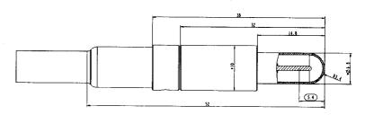
\* add 0.2 mm for tolerance if you intend to make adapters dimensions in mm
