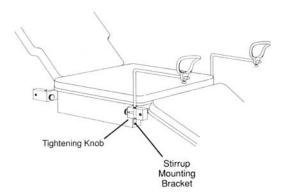
**NOTE:** The portion of the rod with the flat edge should be on the bottom of the horizontal rod.
