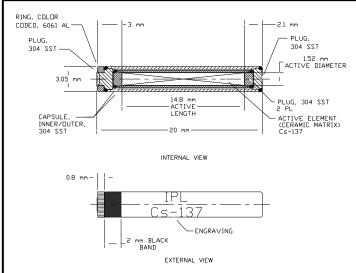
Cs-137 has a half-life of 30.17 years<sup>1</sup> (11020 days) and decays with the emission of characteristic photons and electrons. The stainless steel walls of the tube source absorb the electrons and x-rays. The principal photon emission is 662 keV. The Cesium-137 is absorbed into a ceramic matrix as Cesium Nitrate. Table 1 shows the decay of Cs-137.
