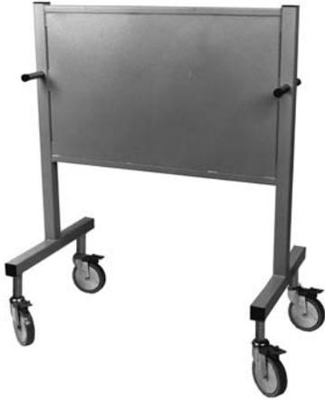
This Rolling Radiation Shield uses 1" thick sheet lead for shielding. It is mounted on a base that has four (4) swiveling and lockable casters which provide easy mobility. The vertical and horizontal posts are filled with lead. The clearance from the bottom of the shield to the floor is 27" so the shield can straddle the CT couch. This shield also has handles on each end to facilitate moving the shield.
