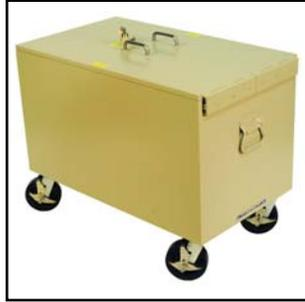
The Shield Box is made of 3/4" (1.92 cm) Steel on all sides, top and bottom which gives a shielding equivalency of 1/4" (.0635 cm) lead.
