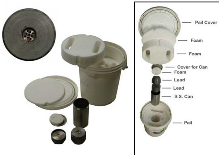
The Cesium-137 DOT Source Transport Pig Container provides for safe temporary storage and transport of up to nine (9) Cesium-137 tube sources. The set consists of a pail with a cover and handle for carrying, foam insert, stainless steel container and cap, lead pig with nine holes for sources and a lead cap. Item 067-650 is for rental only. Rental time is 30 days.
