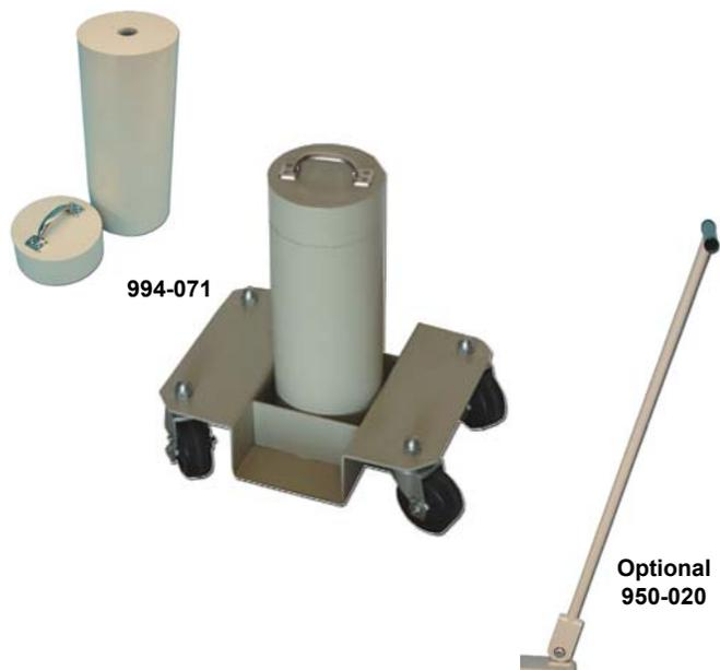
The Lead Storage Container for HDR has a 2" thick (5.08 cm) lead wall and is designed to store the source end of an HDR cable if there is a problem with the retracting system. This container can be easily moved in the cart which has 2" diameter (5.08 cm) swivel casters. The container wall and lid are made of 2" thick (5.08 cm) lead, and the container has an inside diameter of 1" (2.54 cm) and a depth of 10" (25.4 cm).
