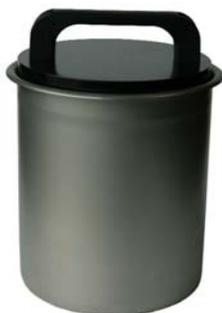
This lead shielded storage container has a stainless steel inner and outer shell. There is 1" of lead between the two shells. The lid is made of 1" thick painted lead and has a plastic handle.
