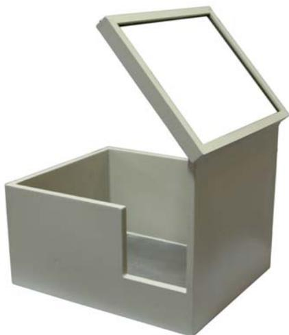
The inside stainless steel bottom is welded on all corner seams to prevent radiation sources or liquids from hiding under any edges or in any cracks, thus, providing easy cleaning. The reinforced steel framework prevents any bending or twisting. One 5/8" (1.59 cm) thick leaded glass piece is inserted into a steel frame with 1/2" (1.27 cm) lead overlapping on the front of the shield.
