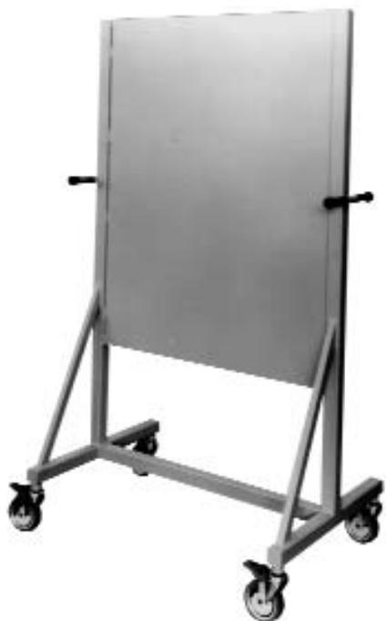
The Fixed Rolling Radiation Shields have a 1" thick sheet lead which will reduce the dose from a cesium source by over 90%. The shield is mounted on a base that has four 6" diameter swivel, locking, ball bearing casters which provide easy mobility. The shield also has handles on each end and side.
