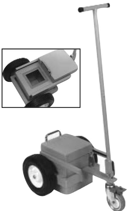
The bottom and sides of the steel container are made of 2" thick lead walls. The sliding 2" thick lead cover (64 lbs.) has a security lock. The steel container has a removable 18 gauge stainless steel liner for easy cleaning. The liner dimensions are 4" sq. x 6" deep.
