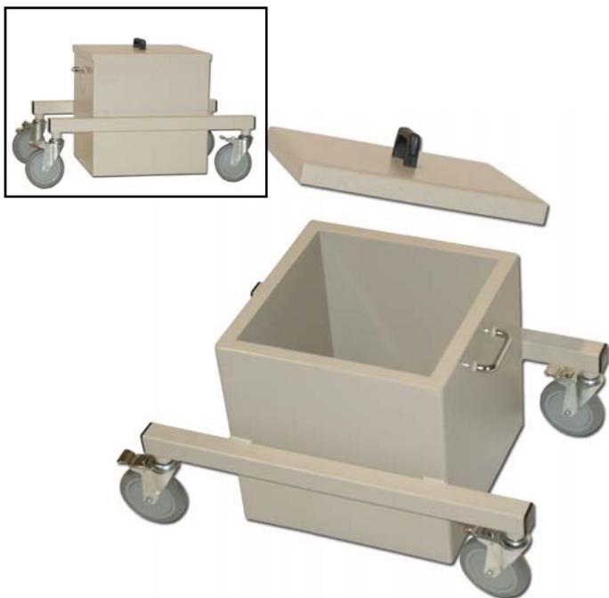
The HDR Cart is designed to store HDR Source Buckets upon arrival to the department before loading into the HDR System. The four walls of the cart have a 1" (2.54 cm) lead thickness. The bottom of the cart and the cover have no lead shielding. The cart has two chrome handles on the sides and the cover has one handle. The bottom of the cart sits 1" (2.54 cm) above the floor. The container is welded to two support bars for the casters. It has four locking swivel casters for ease of moving.
