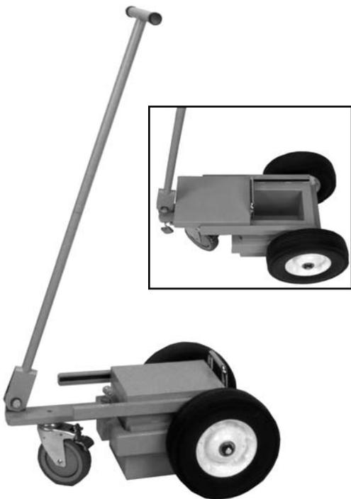
The bottom and sides of the steel container are made of 1" thick lead walls. The sliding 1" thick lead cover has a security lock. The steel container has a removable 18 gauge stainless steel liner for easy cleaning. The liner dimensions are 4 3/8" x 6 3/8" x 5 5/8" deep.
