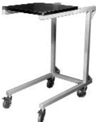
The portable Over Bed Radiation Shield is made of 1" lead covered with stainless steel and mounted on a steel plate which is welded to the top of a tubular steel frame. Wheel extensions on the base provide extra stability when moving.
