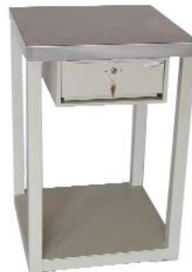
This steel table has smooth, rounded edges with a stainless steel top, a locking storage drawer, and a lower shelf made of 1/8" steel. The support frame is 2" square tubular steel with welded joints for maximum strength.
