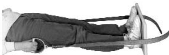
A 'D' style handle is connected to a spring and then to an adjustable leather strap. For easy adjustment, the leather strap has holes every inch and is numbered every fifth hole. The leather strap simply slips over a pin on each side of the foot board.
