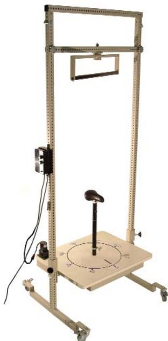
The Rotational Total Body Irradiation Stand was designed for use when treating the total body with electrons.
