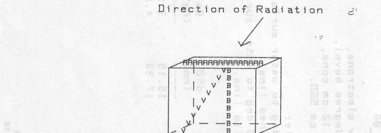
Data is collected in the direction of incident radiation. Direction of scan, number of data points, distance between data points and positioning speed are selectable.
