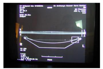
Notice the seven (7) Aluminum BB's shown by the CT image of the alignment bar. When seeing all BB's equally you are assured of proper table (bed) alignment to the CT image acquisition process.
