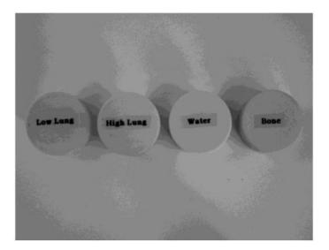
Provides the dosimetry department the ability to quickly to verify the imaging CT scanner is providing correct image values. (Customer to record actual density readings at time of first setup for future caparisoning verifications)
