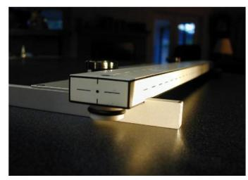
Lateral Laser verification with the alignment bar. Also notice the center dot. Behind this dot on both sides is a Tungsten Pin that the user can take a long port film to check for gantry sag on 90 degree rotation angles.
