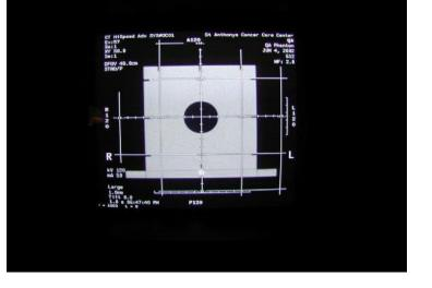
This picture shows the vertical and (left to right) image alignment on scan image reconstruction center. The patient table is centered perfectly left to right.
