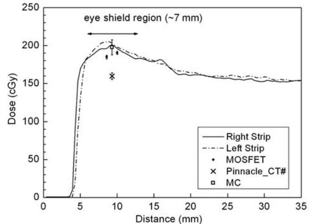
**Fig. 4.** Dose comparison at the inner surface of the eyelid. The MC simulation result shows good agreement with the right EBT2 strip (also with the left EBT2) and superior-inferior MOSFET measurements. The Pinnacle PB calculations on the modified CT images (Pinnacle\_CT#) underestimate the dose by 20%.
