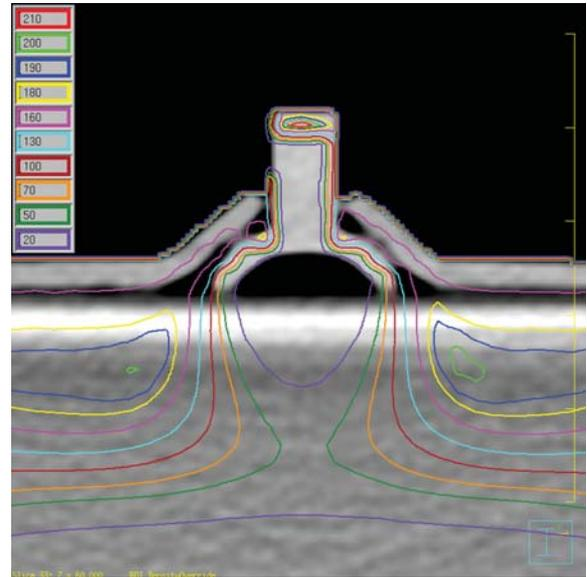
**Fig. 5.** Pinnacle plan results by the contouring and the density override for the tungsten shield and the steel knob. Here, the 0.5-mm thickness of the aluminum cover assembly was not considered.
