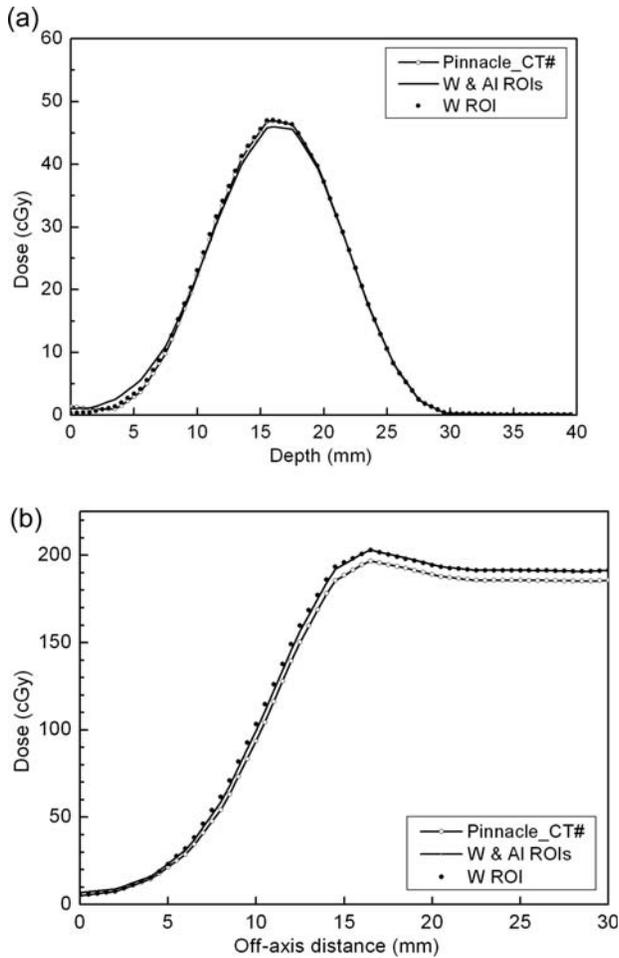
**Fig. 6.** (a) Pinnacle central depth profiles for the modified CT (Pinnacle\_CT#), contouring of the tungsten shield/steel knob/aluminum cover and density override CT (W & AI ROIs), and the aluminum cover-neglected CT (W ROI). (b) Lateral profiles for the same CT data sets. Consideration of the thin aluminum cover does not make any practical differences to the Pinnacle calculation.
