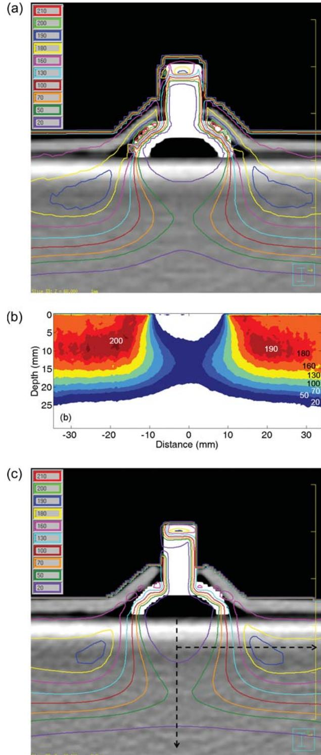
**Fig. 2.** (a) MC simulation results with the modified CT images at the isocenter plane. (b) The EBT2 film results below the eye shield. Legends for dose values are added. (c) Pinnacle plan results with the same modified CT images. Analysis was conducted for the right half, assuming symmetric.
