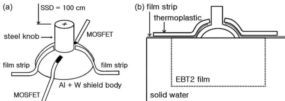
**Fig. 1.** An experimental setup. (a) Two EBT2 film strips on the right and left sides, two MOSFET detectors on the superior and the inferior sides, covered by 3-mm thickness thermoplastic for an eyelid simulation. The beam isocenter is at the top center of the steel knob. (b) A vertical EBT2 film is sandwiched with solid phantoms under the eye shield for the dose distribution measurements.
