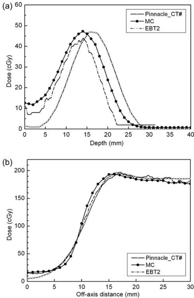
**Fig. 3.** (a) Central depth profiles and (b) Lateral profiles from the modified CT-based Pinnacle plan (Pinnacle\_CT#), MC simulation, and EBT2 film measurements. Along the vertical and the horizontal dashed lines in figure 2(c), profiles were extracted.
