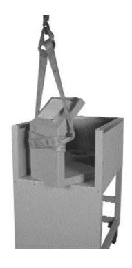
When Lifting the 450 lb, "L" Block use a sling and a 7/8" dia. x 21" long steel bar. Wrap sling around "L" Block and then around steel rod so when unit is lifted it only tilts a small amount. Bring "L" Block into Work Station at 45° so steel bar can be removed. Remove sling and steel bar, then slide unit into position.
