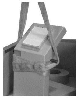
View of sling wrapping and steel bar for lifting. The steel bar is slid through the two holes in the "L"-Block.
