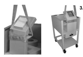
**3.** View of sling wrapping and steel bar for lifting. The steel bar is slid through the two holes in the L-Block.
