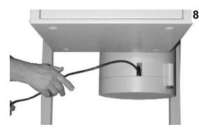
8. Rotate bottom well cover back in place. Making sure not to damage the cord on the dose calibrator.
