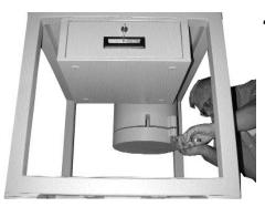
4. Remove (1) bolt ONLY securing well shield base cover. Removing both bolts may result in serious injury. Loosen 2nd bolt 1/2 turn so the cover will rotate.
