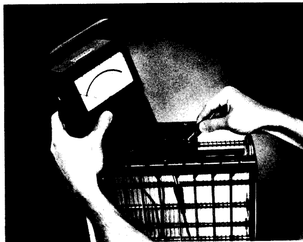
USE AN OHMMETER TO CHECK THE ELECTRONIC CELLS FOR SHORT CIRCUITS
