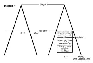
The doses are normalized to  $d_{max}$  without the eye shield (Diagram 1) using a 10 x 10 cone. When 1.00 Gy is delivered to  $d_{max}$  using 6 MeV with the shield, you get 1.08 Gy to the undersurface of the eyelid (Point 1) and 3.4% transmission to the lens (Point 2) (See table 1).
