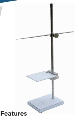
This system will calibrate all optical distance indicators on accelerators, cobalts and simulators. The ball pointer is used to determine the rotational isocenter of the treatment machine collimator head and gantry. The ball pointer is also visible in fluoroscopy on simulators.
