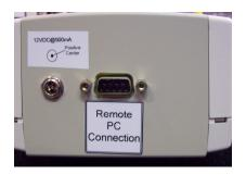
To connect the remote to the area monitor place the DB9 male connector from the supplied cable into the connector on the bottom of the area monitor marked Remote/PC connection. Tighten the two screws to secure the connector to the area monitor. Connect the other end of the cable to the remote and secure.
